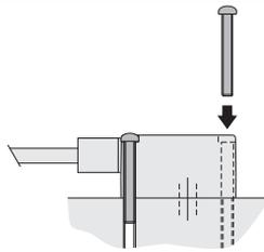
Use the small screws provided to mount the sensor head.
