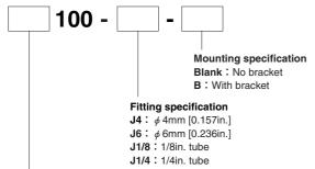
$\ensuremath{\mathbf{FN}}$  : Air filters for pressure and vacuum
