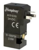
The **A15 Series** (shown actual size at left) is 15mm in width, produces 0.05 Cv flow, power consumption of only 2.5 watts, and is available in standard DC voltages of 12V and 24V. Valves are available normally closed or normally open (to 100psi), electrical entry of lead wire or mini-DIN, including fluorocarbon seals, along with a non-locking override.
