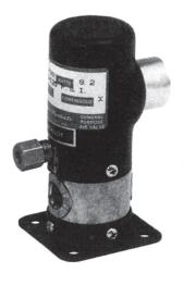
250E2 250AE2-3-21 Model 250E2 is a double-solenoid, momentary-contact, maintained-position, 2-way or 3-way valve. It holds in either the closed or open position with internal air pressure.
